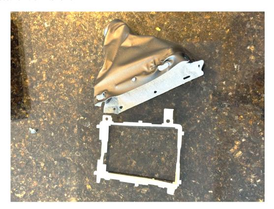
7. Turn the boot inside out and remove the plastic ring.
