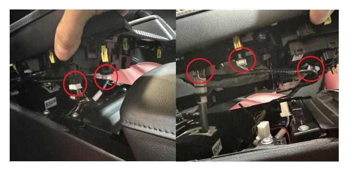
5. Remove the 2 Phillips screws (red) and pull the white plastic frame/boot assembly out of the console.
