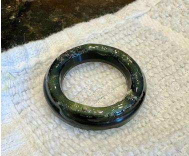
9. Place the ring over the boot, pressing it in place around the perimeter of the ring, and turn right side out.
