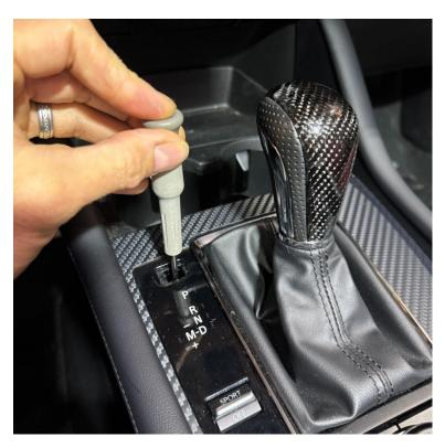
2. Insert a tool (a small flat head screwdriver works) and move the tool in the direction of arrow (1) to detach the hook. Move the lock release button cover in the direction of the arrow (2) and remove it.
