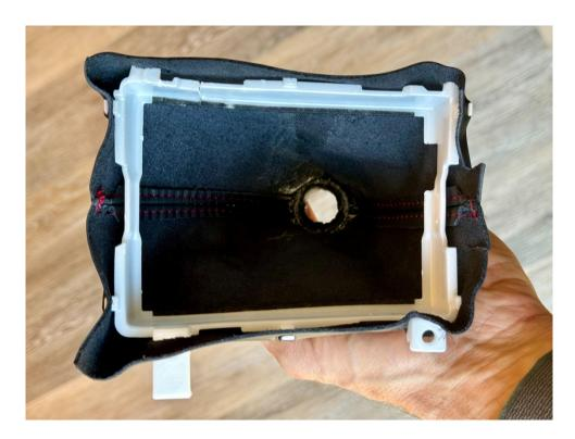
11. Place the boot assembly back in the console, screw the two screws back in, and reinstall the console in the car, being sure to plug all four connectors back in.
