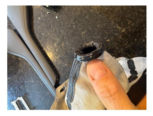
8. Turn the new boot inside out. Place cement on the ring and the upper perimeter of the boot.
