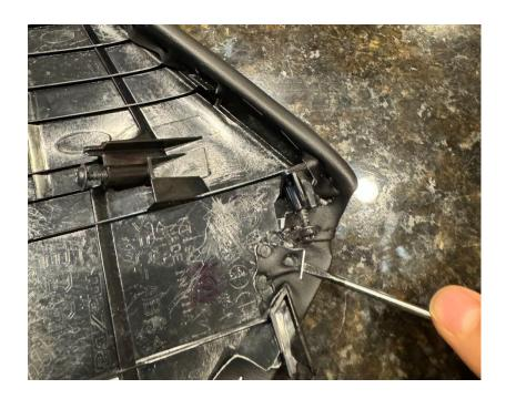
9. new piece and the base piece out on a table and put a layer of adhesive along the black unfoamed line of the base piece and the stitching on the backside of the leather. Don't go too thick here, you don't want adhesive seeping through the seam.
