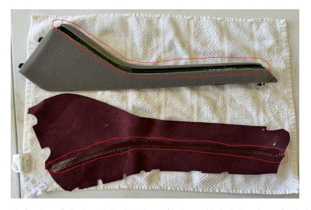
10. Put a layer of adhesive on the interior perimeter of the base and the backside perimeter of the leather. Then work your way around the perimeter, pulling tight and sticking the edges in place. Some trimming may be necessary.
