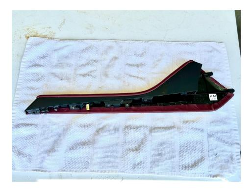
12. Attach both side console pieces to the main console and reinstall in the car, being sure to plug all four connectors back in.
