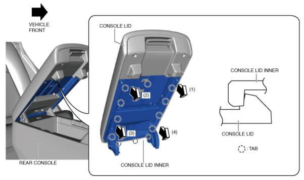
3. Using a remover tool or pulling carefully, move the console lid lock in the order of arrows (1), (2), (3), and (4) shown in the figure, detach the tabs, and remove the console lid lock.
