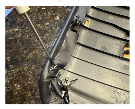
5. Lay the cover and armrest upside down on a table. Place cement around the perimeter of the cover and the armrest. Make sure the cover is centered, push down firmly on the middle of the armrest, and work your way around, pulling tight and sticking the cover to the armrest. Make sure any slits in the leather are secured over the plastic tabs.
