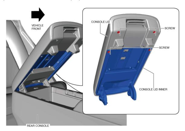
2. Using a remover tool or pulling carefully, move the console lid inner in the order of arrows (1), (2), (3), and (4) shown in the figure, detach the tabs, and remove the console lid inner.
