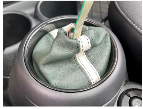
9. Install the shift handle, connect the ribbon cable, and attach the lower face plate.
