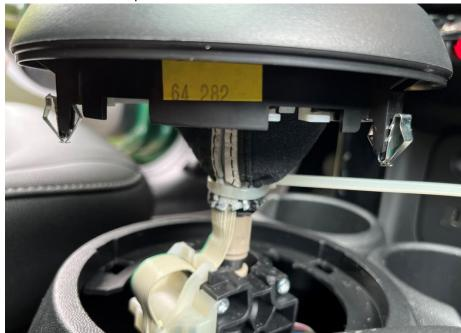
11. Snap the trim ring back into place and snap the front face plate back together.
