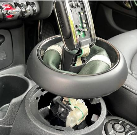
10. Lift the outer trim and place a zip-tie around the boot and the shift handle. The handle can then be slide down until it clicks into place.
