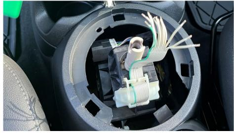
6. Remove any remaining boot material from the large trim ring. Note which side is toward the front of the car. The ring can only go in 1 way.
