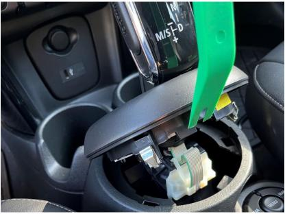
4. Like a manual shifter, you could pull the shifter off, but if you do, it will likely destroy the ribbon cable. Instead, use a screwdriver or other tool to pry the shift handle up slowly, just to get it disconnected from the shifter.
