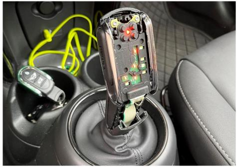
2. Disconnect the ribbon cable from the circuit board.
