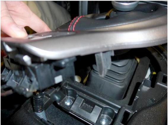
Now, disconnect the switch connector and stretch the boot over the reverse lockout to remove it.
