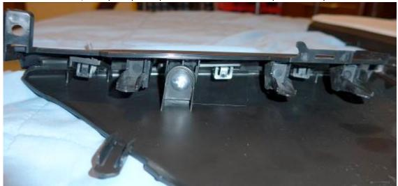
Use a suitable glue to attach the foam to the knee pad.
