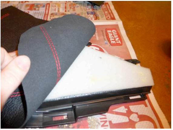
Trim the edges of the leather so it will wrap around the edge of the pad without interfering with any of the mounting tabs.
