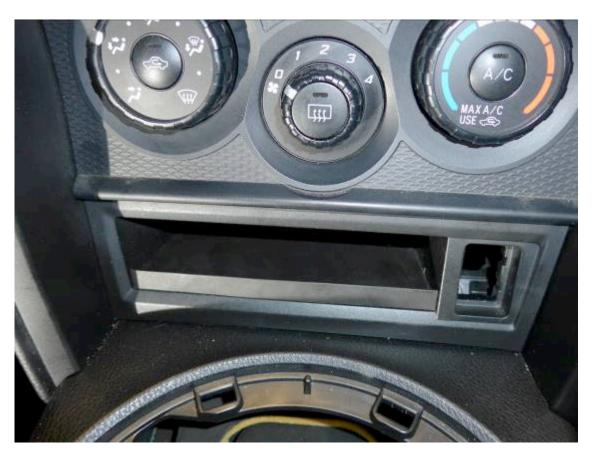
Remove the last two screws that hold the console in place, then remove the console from the vehicle. Remove the connector to accessory power as you do.
