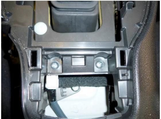
To gain access to the last two screws, you need to remove the tray below the climate controls. Start by pulling off the lower trim piece under each kneepad.
