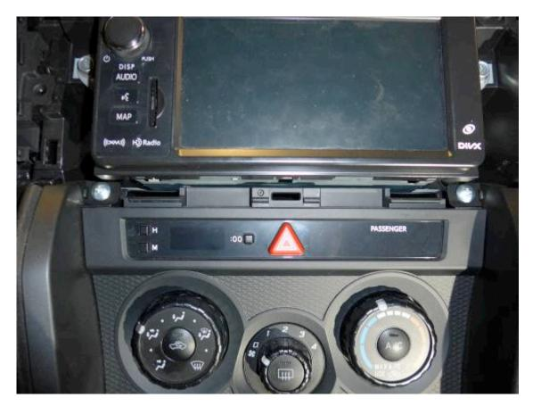
Remove this screw, then pull up to separate the inner and outer parts of the pad.
