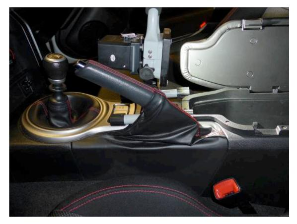
The shift boot comes off next. First, twist off the shift knob. Then, use a trim tool to separate the silver trim piece from the console.
