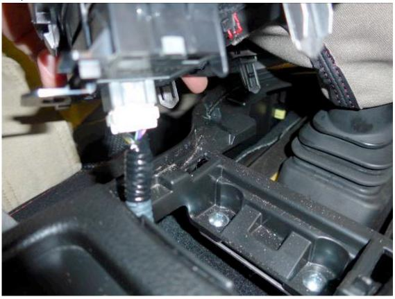
Now you can remove the center two screws that hold the console in place.
