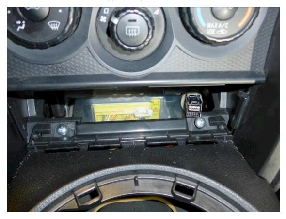
Use a trim removal tool to remove the piece around the radio, then remove the screws (1 each) that hold the knee pads in place. Pull the knee pads straight toward the back of the car to remove them.
