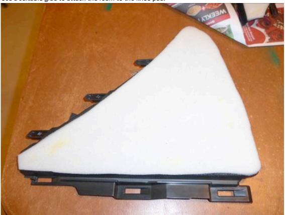
Place the leather on top of the pad, lining up the stitching where you want. Working in sections, glue the leather to the foam.
