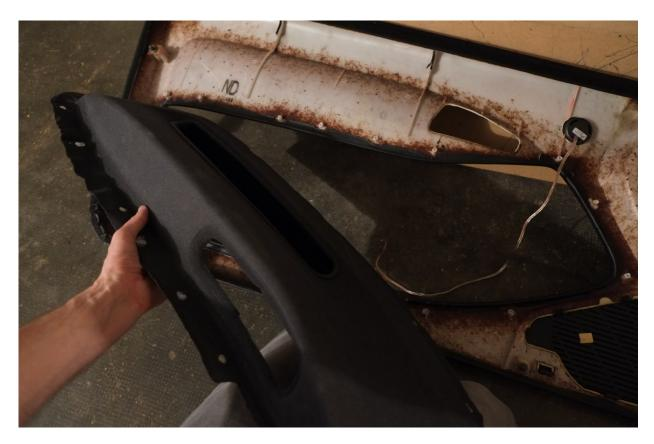
Now remove the black plastic part starting with the three rear screws.
