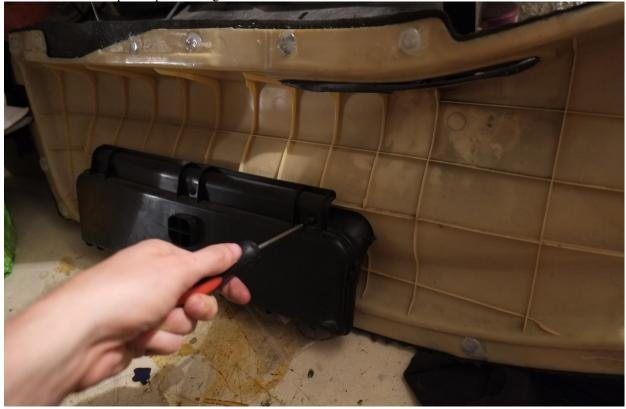
The rear side is old with two clips on the two sides. Care when you unplug it, they are a bit weak.
