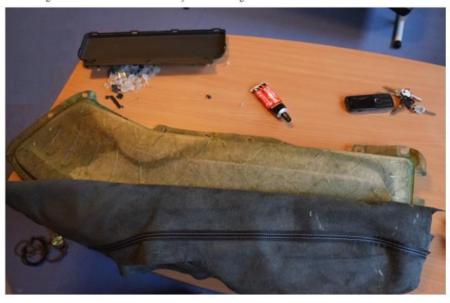
On corners of the door, the fabric should be taut and absolutely must keep the position you give it.
