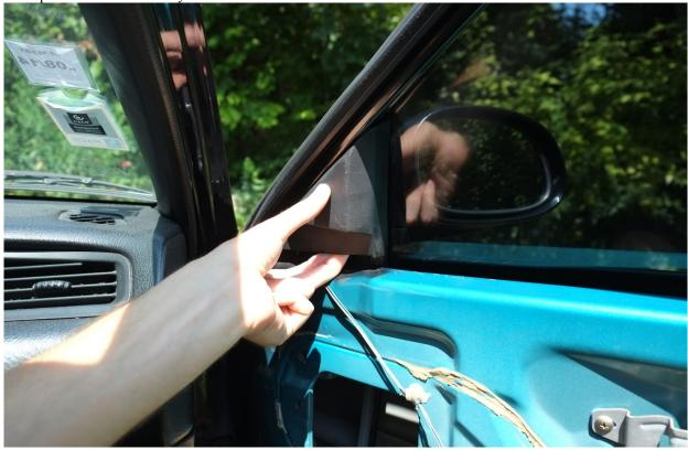
Reattach the trim in the same way that you removed, taking care to re-clip all the edges on the door side. Then replace,
