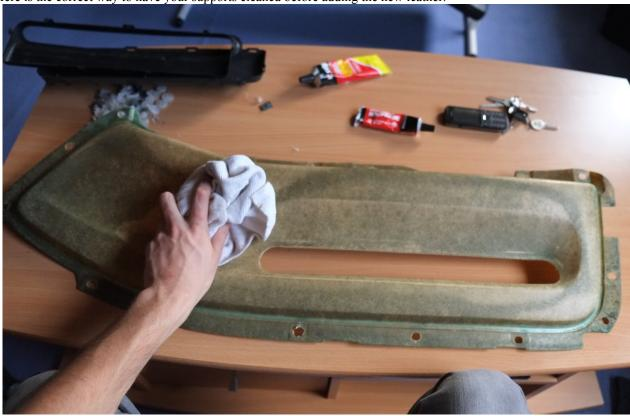
You can now place your new fabric and correctly position on the liner. Take care of fixing it well in the corners in order to be in its final position.
