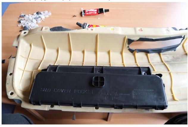
Reassemble the plastic lower storage and don't forget to cut the fabric all around the holes
