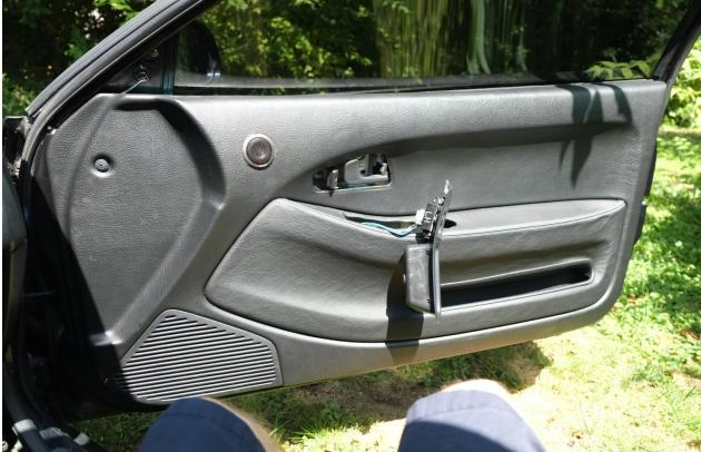
Finally, reassemble the door handle by screwing the cover.
