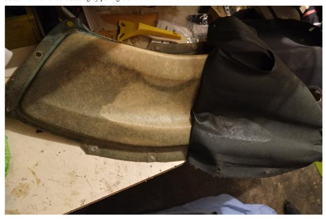
If necessary you have to correctly empty the glue hole because residues can prevent cored bond when you reinstall the panel back into the car.
