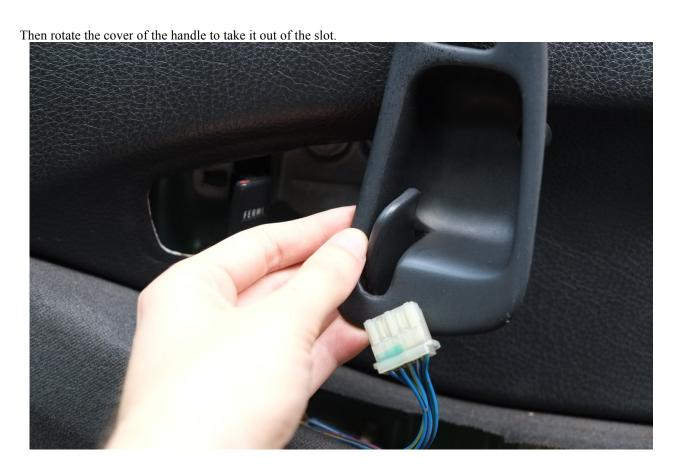
Now you can remove the door panel. Start by pulling the door panel to unclip it from the door. There is approximately 10 clips around the door. Start with the bottom left side, easier side to unclip.
