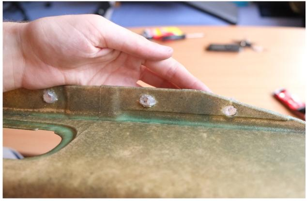
Here is the correct way to have your supports cleaned before adding the new leather.
