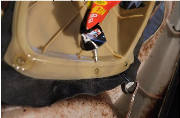
Let dry for a full day before remount the door panel. Then proceed to reassemble the door. For convenience, remove first the plastic cover mirrors if you have not done it before.
