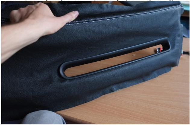
Then screw the plastic back to the armrest, the fabric cannot move anymore so it will be easier to glue it properly to the other parts of the door.
