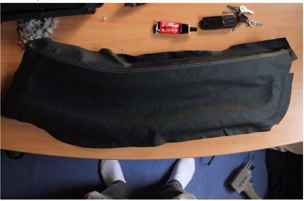
Carefully cut the fabric in places where the plastic door must be reattached. Make sure to leave enough margin. You can always trim off more when necessary. An X-acto knife is the best tool for this purpose.
