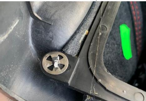
11. The emergency brake boot is held by 3 circle fasteners and a metal bracket. Using the same method as step 11, remove the 3 circle fasteners. No need to remove the metal bracket, push bottom of shift boot off the bracket and remove.
