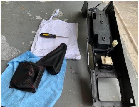
10. The shift boot is held on by 4 circle fasteners, use flat head screwdriver to gently pry these off of the plastic, work around each side until the circle fastener is removed. Repeat on 3 other fasteners.
