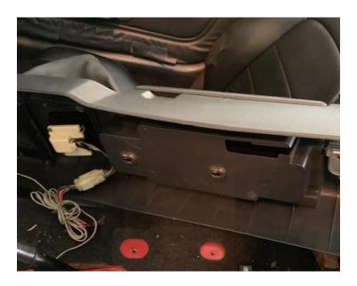
8. Disconnect the connector for the window controls, and disconnect the connector for the interior light.
