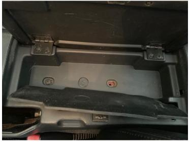
2. Remove 2 front screws on either side of the console, just below the shifter.
