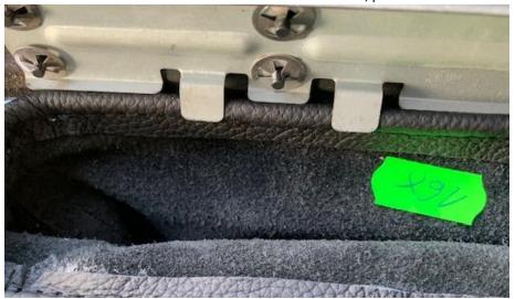
12. To install shift boot, place new shift boot in place and push plastic guides through each hole, fasten down with the circle fasteners. Push down the circle fasteners with a flat head screwdriver to ensure they are properly seated.
